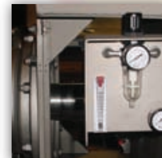
Air purged seals with flow meters and F/R/G
