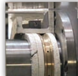
Air purged packing gland seal with split housing
