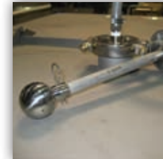
Tri-clamped ferrule with removable spray ball for CIP cleaning
