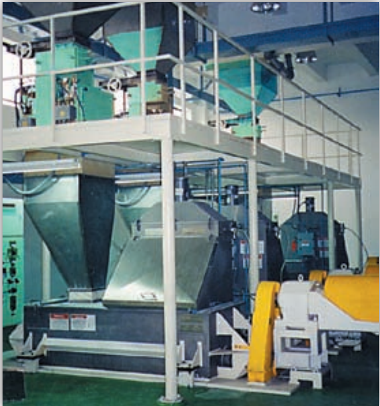
Value added sugar processor with scaling of major ingredient and filtered bag dump for minors
