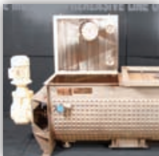
ASME dimple jacketing for heating or cooling
