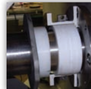
Split, removable packing gland seals with Teflon V-Rings, suitable for USDA dairy applications
