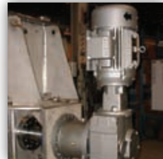
Direct drive, right angle shaft mount
