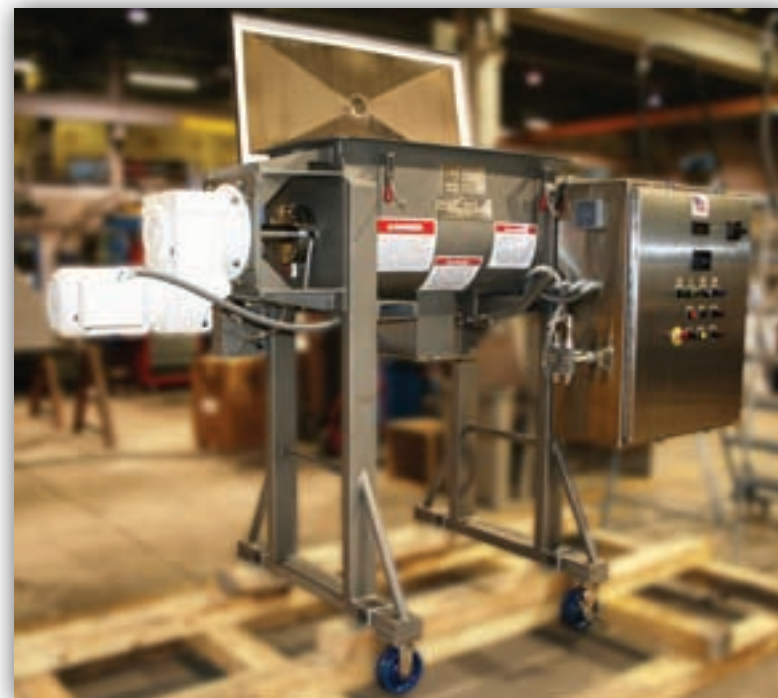
Direct drive, right angle shaft mount
