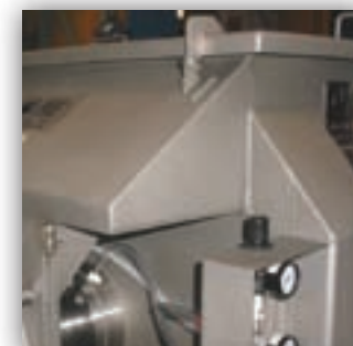
Shrouded endplates for easy cleaning
