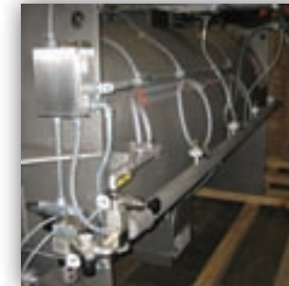
Compressed air header to seals and discharge valve and NEMA 4x SS J-box for single phase components
