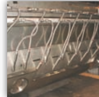
CO2 tangentially mounted injection nozzles and manifold
