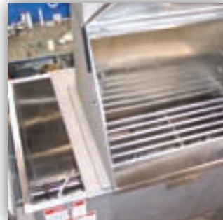
Dust controlled, easy clean, tailored blender cover
